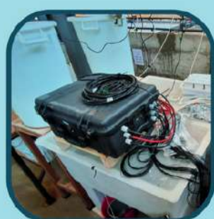
RAFT VALVOMETRY EQUIPMENT
